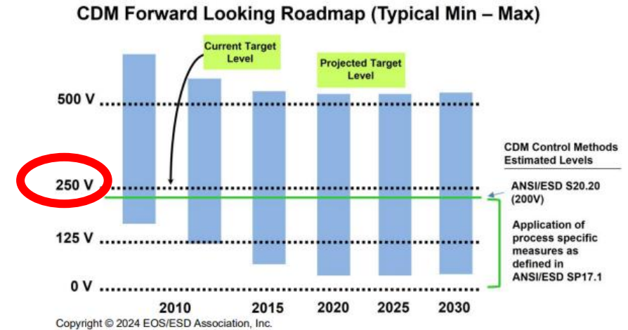
Figure 4: 2010 to 2030 Charged Device Model Sensitivity Limits Projections NOTE: The current target level is 250 Volts.
