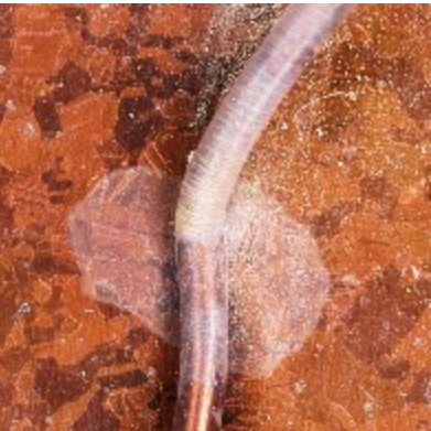
Crack & Delamination in Parylene Coating on Cu-AMB
