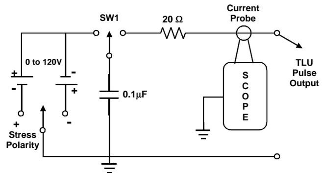
Figure 1: First generation dual-polarity TLU pulse generator
