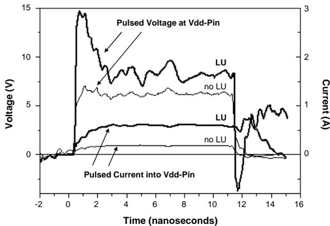
Figure 20: Pulsed voltage and current at DUT pin under test
