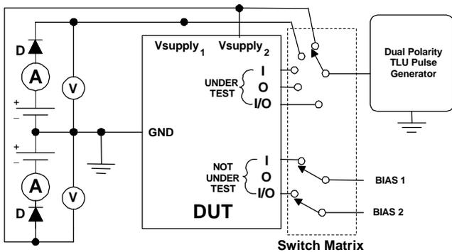
Figure 3: Typical TLU test configuration
