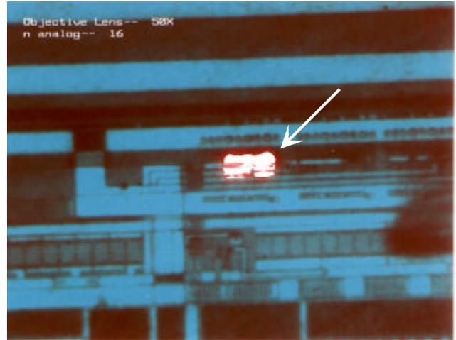
Figure 12: Photo-emission site during RC TLU latch event
