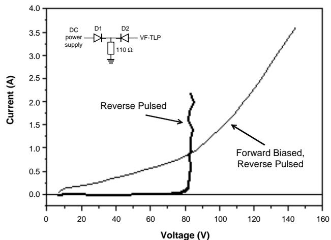
Figure 8: I-V reverse breakdown curve of a pulsed LL101 diode (D1)
