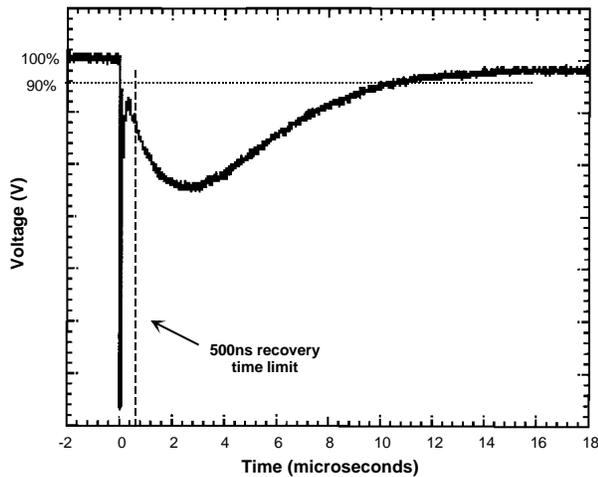
Figure 15: PSR test for automated TLU simulator without booster circuitry; note effect of internal wiring/cabling on response
