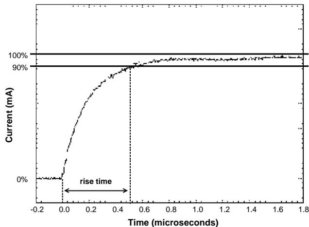
Figure 6: PSR test; power supply current response
