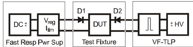
Figure 19: Test configuration for VF-TLP transient latch-up
