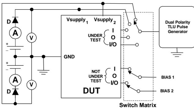
Figure 3: Typical TLU test configuration
