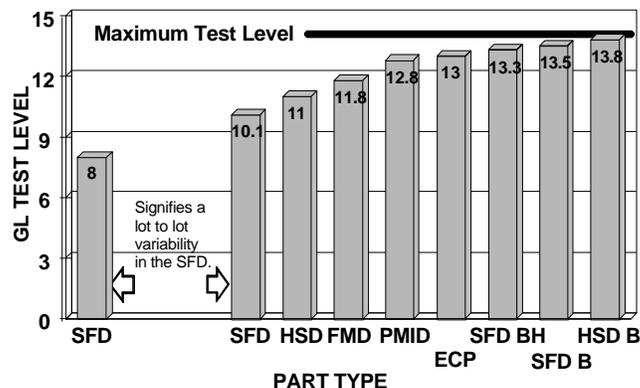
Fig. 6 Relative part resistance to GL.
