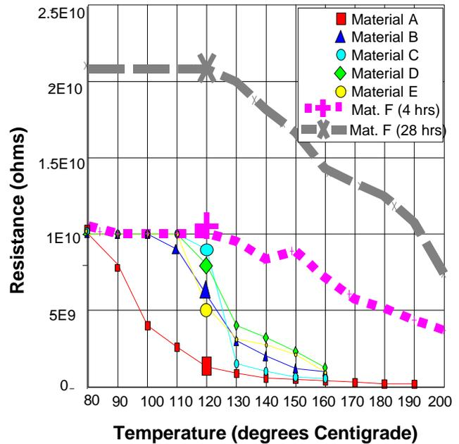
Fig. 5 Material resistance change with temperature.
