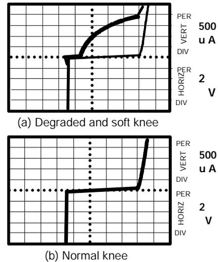
Fig. 2. The characteristic curves of an input pin exposed to and degraded by GL
