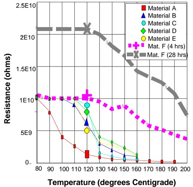
Fig. 5 Material resistance change with temperature.
