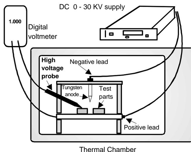
Fig. 4. GL test fixture and equipment.
