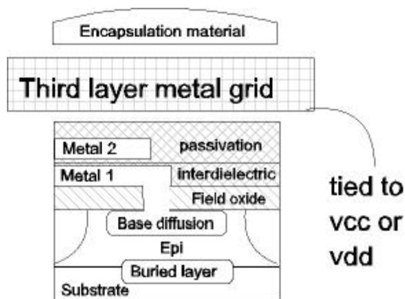
Fig. 3. A typical dual metal part with a third layer metal grid.
