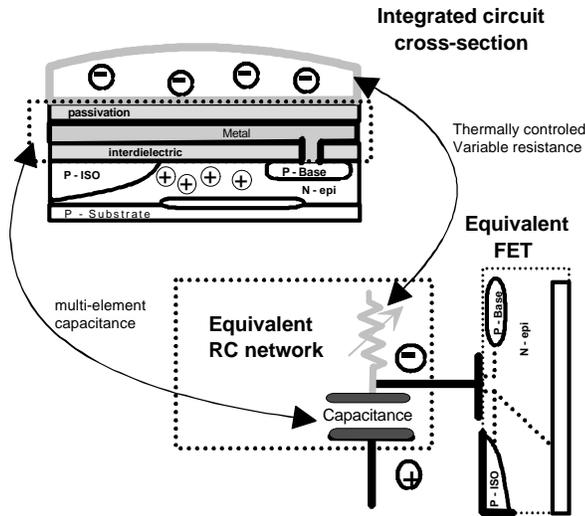
Fig. 1. Cross-section of a dual metal circuit and the equivalent GL circuit.
