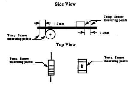
Figure 1 Leaded and Surface Mount Device Temperature Sensor contact points
