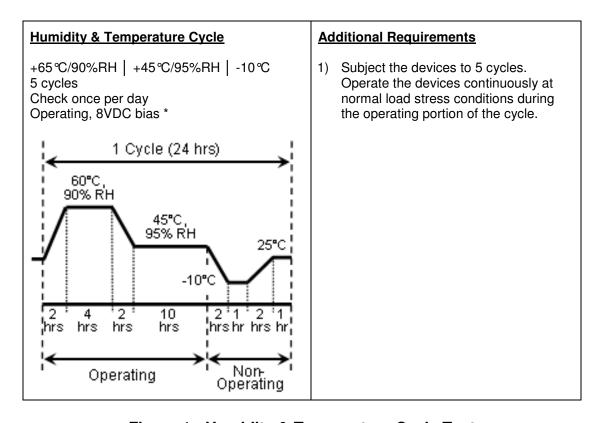
Figure 1: Humidity & Temperature Cycle Test
