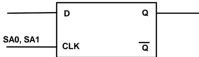
Figure 15: CLK faults will be detected if SA0 and SA1 faults are detected on D or Q
