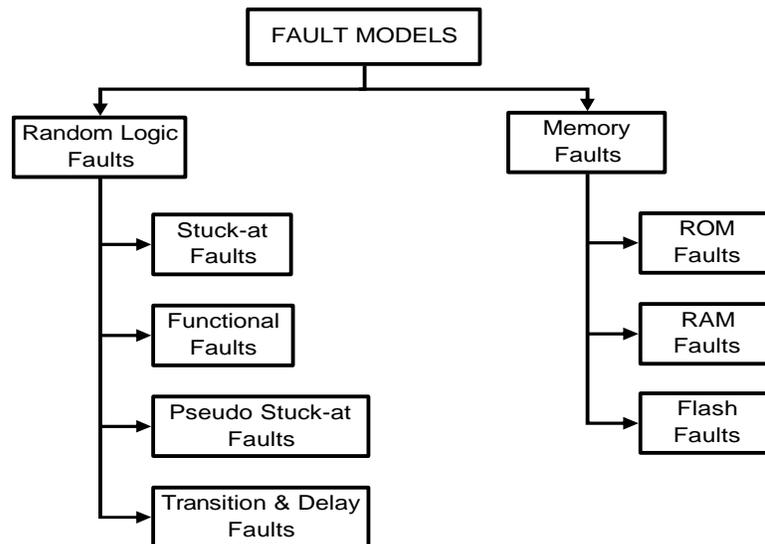
**Figure 4: Fault Models**
