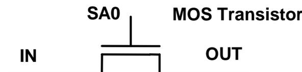
**Figure 14: Control SA0 will be detected if (OUT) SA0 and SA1 faults are detected when no other sources fan-in to signal OUT (Implied Fault Detection)**
