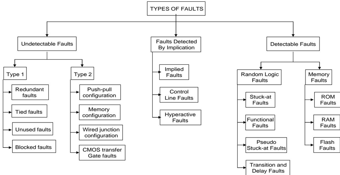
**Figure 3: Fault Types**
