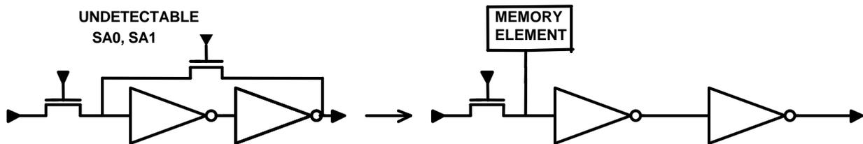
Figure 11: Undetectable Faults in a Memory Configuration
