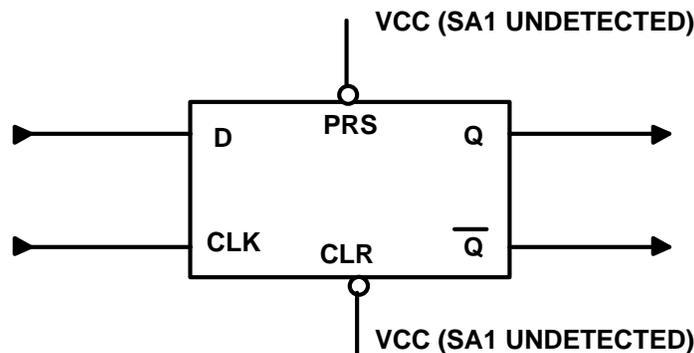
**Figure 8: SA1 on both inputs is untestable tied**
