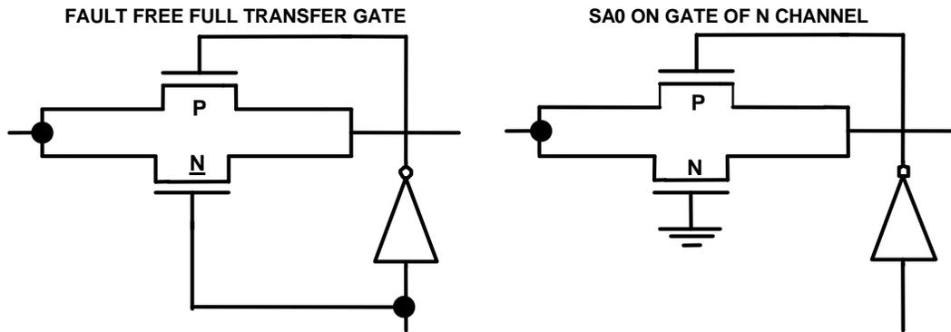
**Figure 13: CMOS Transfer Gate Undetectable Fault - Circuit Fault Effect**
