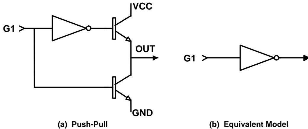
Figure 10: Push-Pull Configuration
