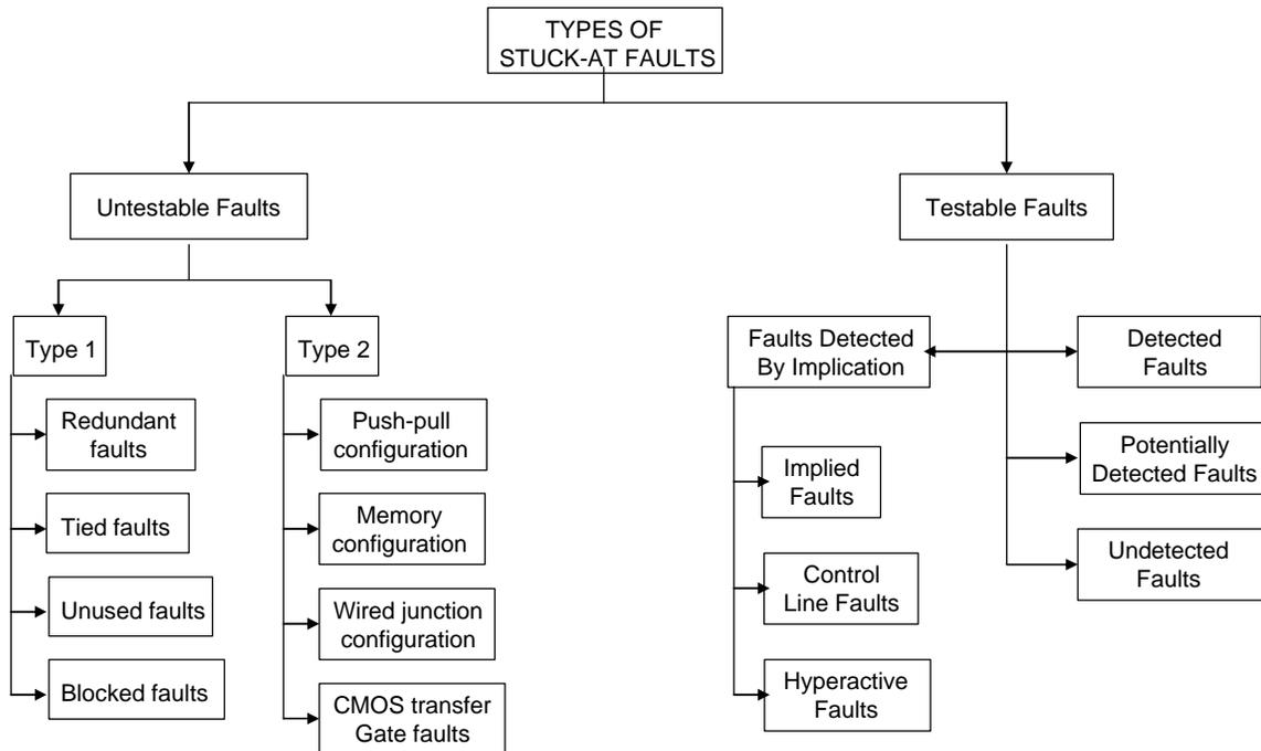
**Figure 6: Types of Stuck-at Faults**
