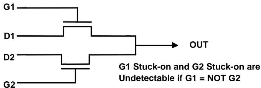
Figure 12: Undetectable Fault in a Wired Junction Configuration
