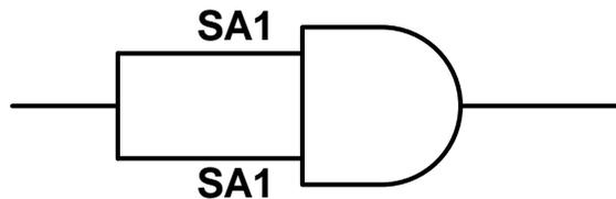
**Figure 7: SA1 on either one of the inputs is untestable redundant**
