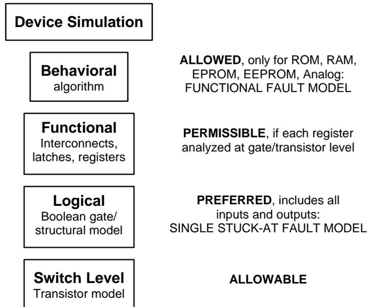
**Figure 2: Device Simulation for Integrated Circuits**
