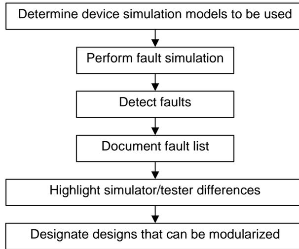
**Figure 1: Typical Fault Simulation and Fault Grading Procedure Flow**
