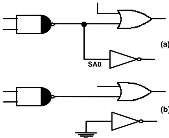
Figure 5: (a) Fan-out Logic (b) Same Logic with SA0
