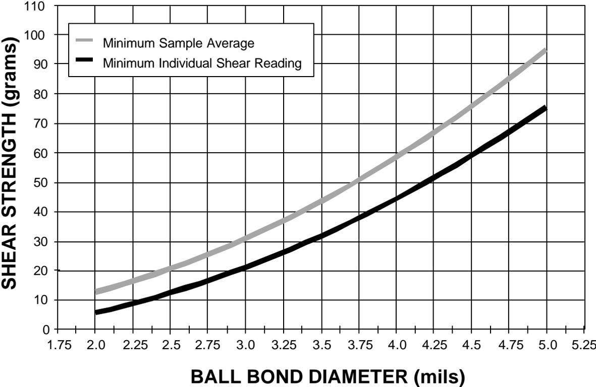
Figure 4: Minimum acceptable individual and sample average ball bond shear values \*, see Table 1 for exact ball bond shear values \*
